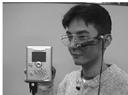
Fig.10: New hearing assistive device with a speech recognition and a see-through HMD
