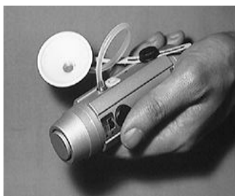
Fig 4 : Manufactured electric larynx
