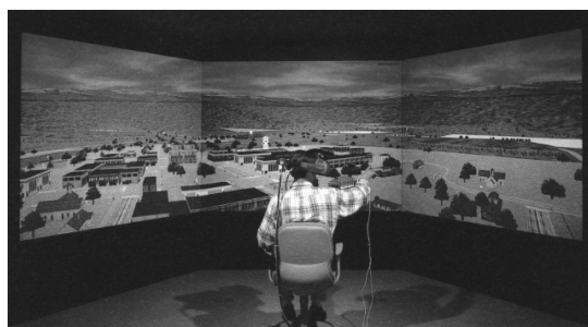
Fig.13 Arch-screen and a motion base with two force plates equipped inside the MR system laboratory
