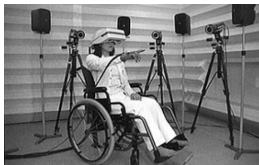
Fig.12: Speaker array for displaying virtual obstacles
